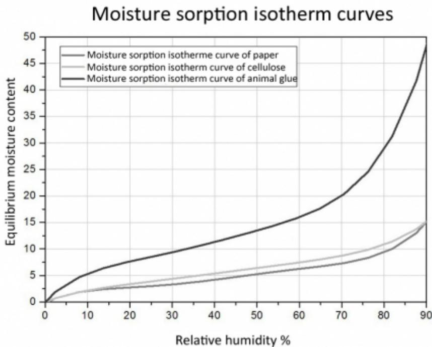
Water-vapour balance between humid air and hydrophilic materials. Roche A., 2016, p.51.
